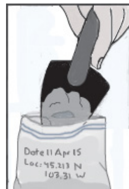
Figure 3. Place the soil in a sealable plastic bag.
