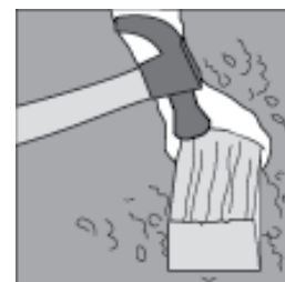
Figure 6. Gently tap the sample can with a wood block and hammer.
