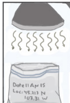
Figure 8. Dry the soil under a heating lamp.
