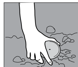
Figure 4. Push the sample can into the soil.
