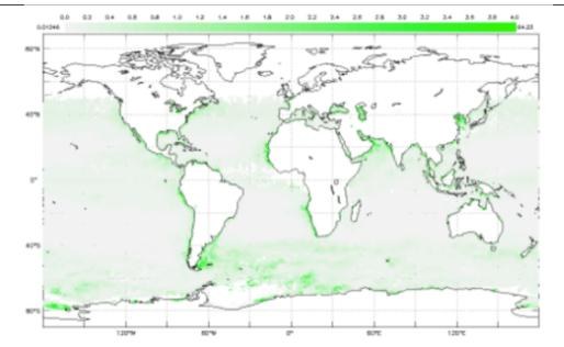
• Monthly Flow of Energy into Surface by Shortwave Radiation (watts per square meter) - This quantity describes the total flow of energy from the Atmosphere to the surface by shortwave radiation, which is the visible light coming from the Sun. This is the flow of energy that warms the Earth's surface during the daytime. Clouds affect the rate of this energy flow, and the rate also varies with the seasons (higher rate in summer and lower rate in winter).
