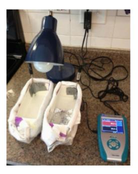
• Sample results from Carbon Dioxide and Air Temperature Lab, set up as pictured below: (200 watt light bulb, about 20 cm from the cups)
