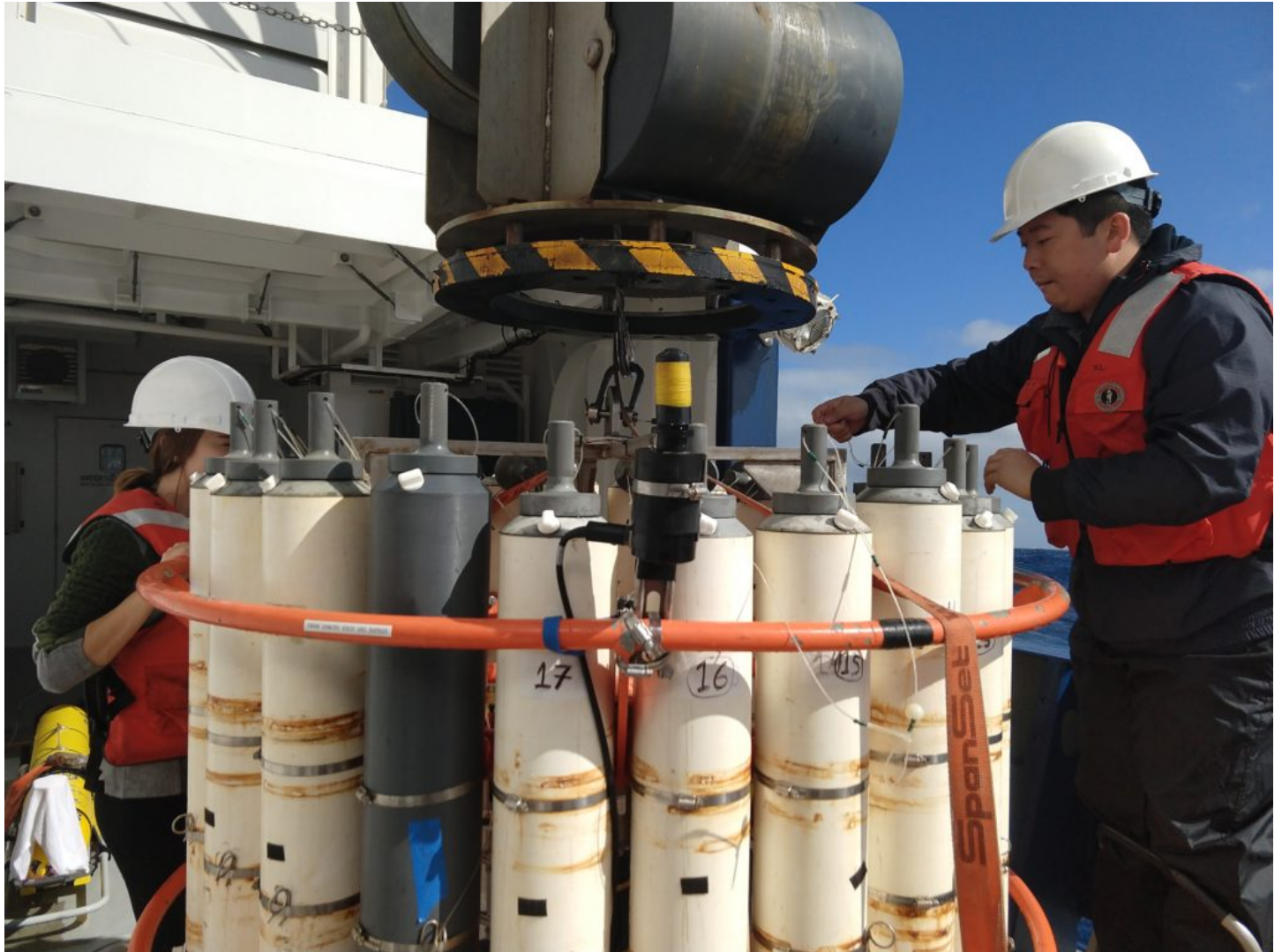
Scientist Yuanheng Xion cocks niskin bottles before our test Conductivity, Temperature, and Depth
